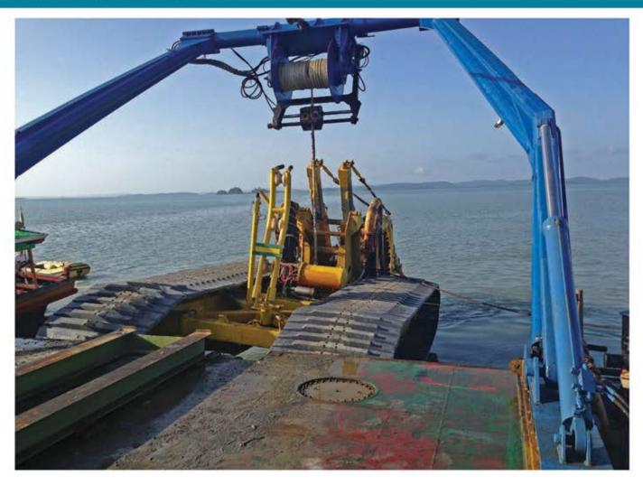
SEA specializes in trenching various types of cables (i.e. FOCs, umbilicals and power cables) during and/or after the the laying operations,
