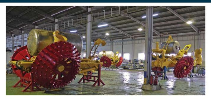
SEA pioneered the "post-trenching system" for the burial of pipelines and cables.
